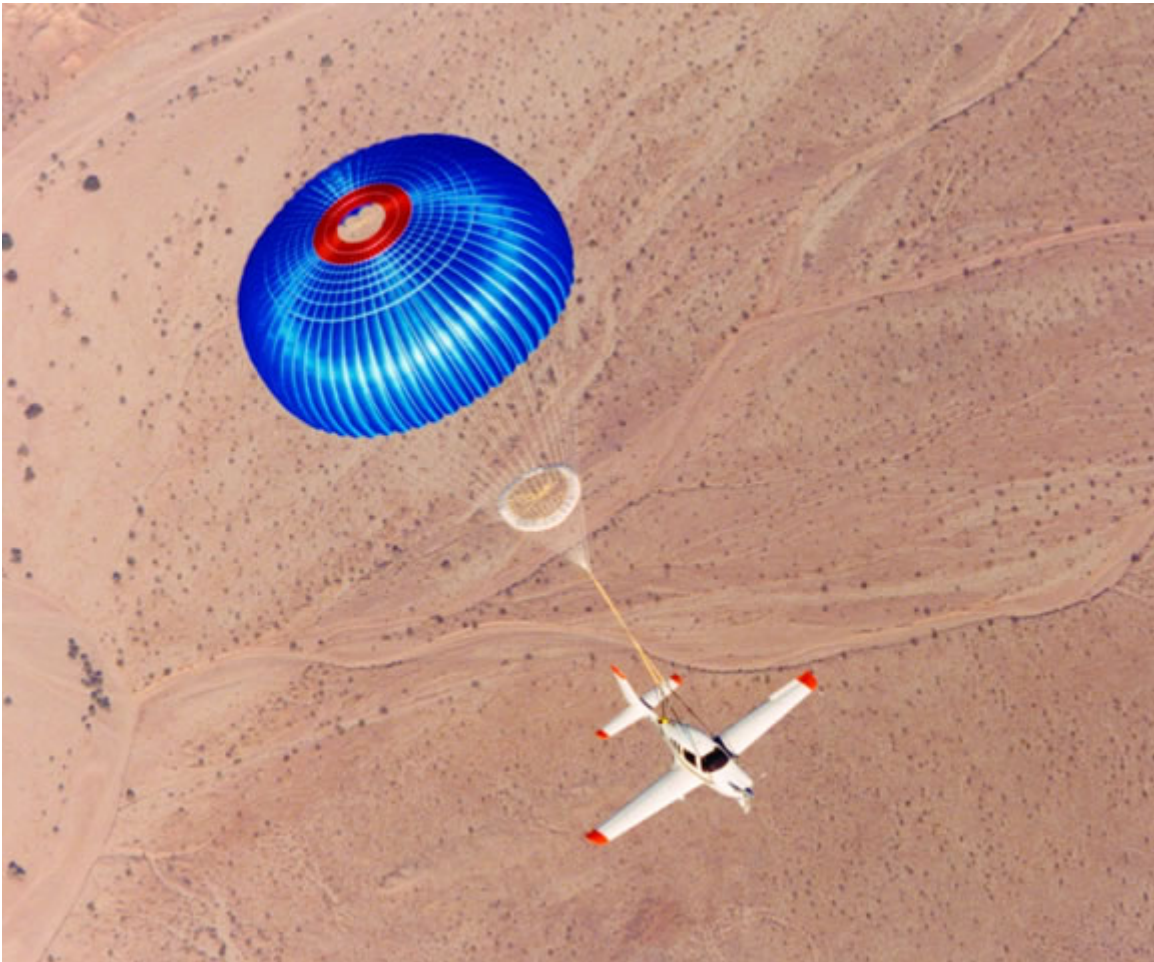
Cirrus' signature parachute will also be a feature on the small jet
