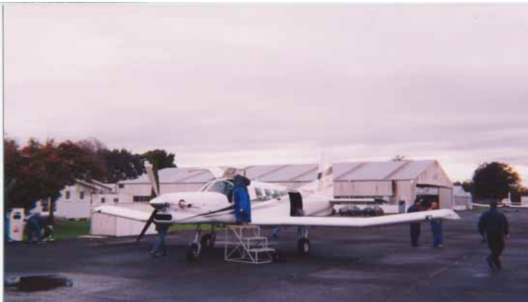
PAC 750 powered by PT-6, world's first purpose built parachuting aircraft
